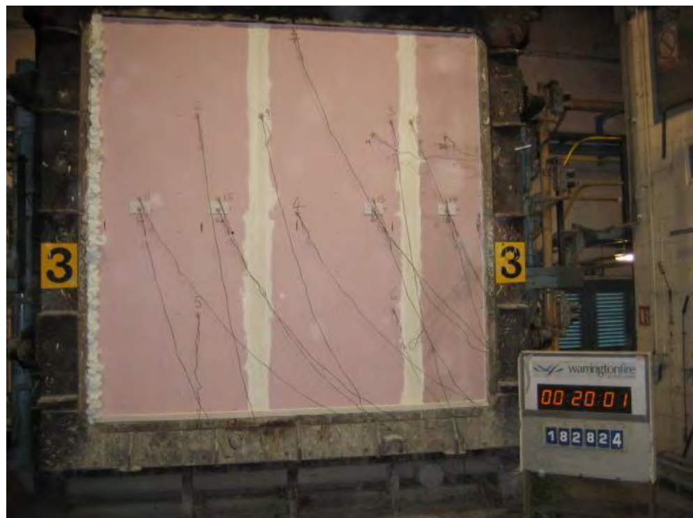
The unexposed face of the specimens after 20 minutes of testing
