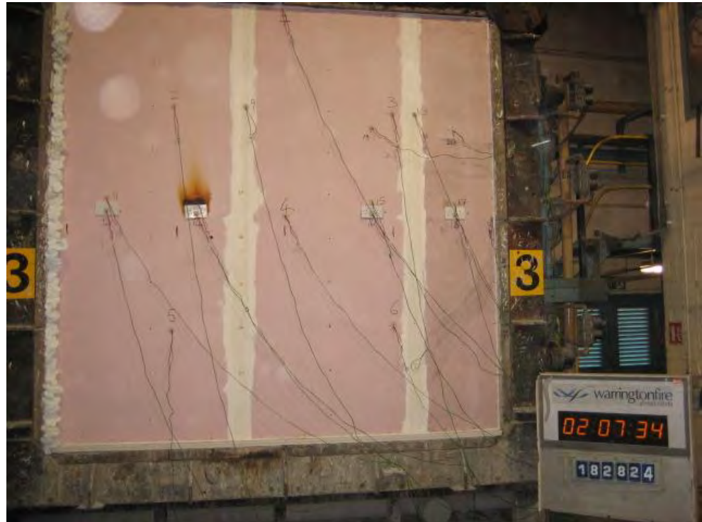
The unexposed face of the specimens after 127 minutes of the test
