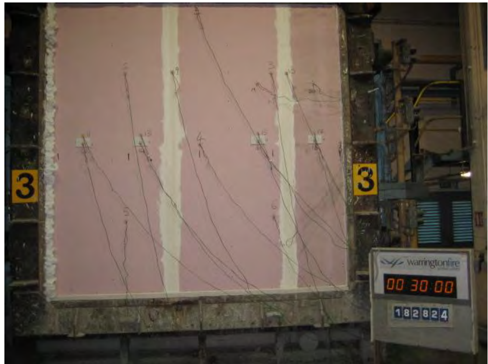
The unexposed face of the specimens after 30 minutes of the test
