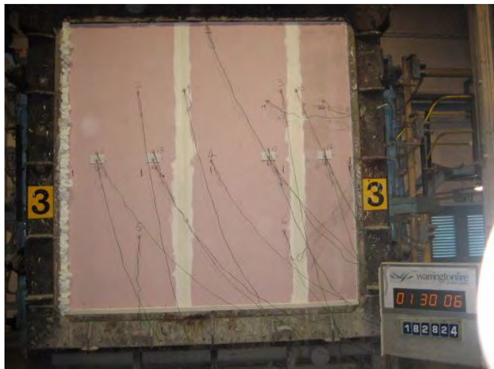
The unexposed face of the specimens after 90 minutes of the test
