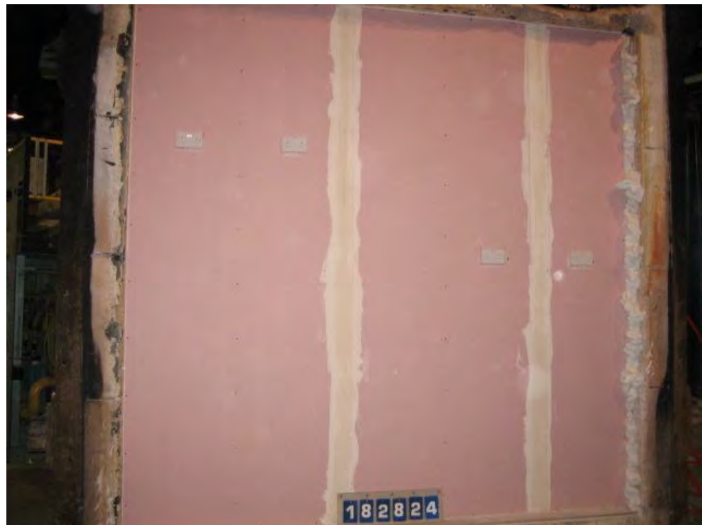
The exposed face of the specimens prior to testing
