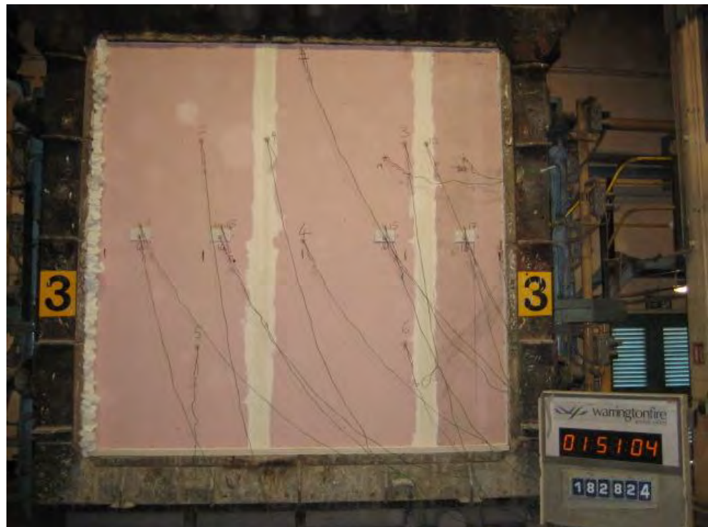
The unexposed face of the specimens after 111 minutes of the test
