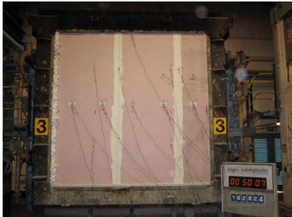
The unexposed face of the specimens after 50 minutes of the test
