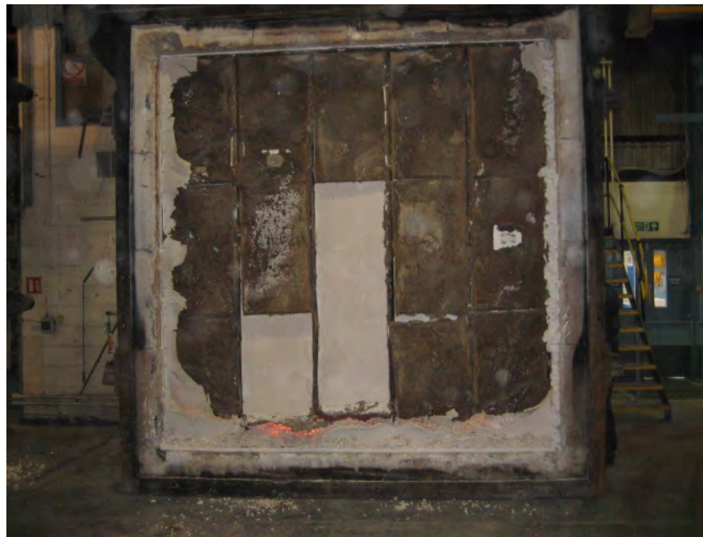
The exposed face of the specimens shortly after testing
