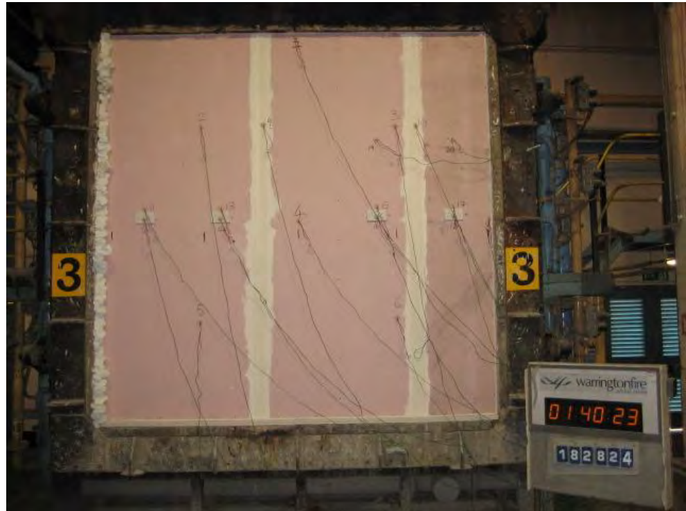
The unexposed face of the specimens after 100 minutes of the test
