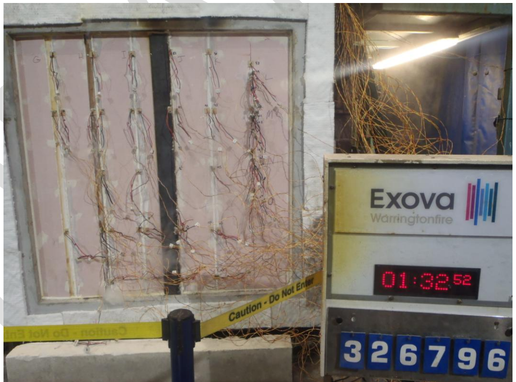
The unexposed face of the wall construction after 92 minutes of testing
