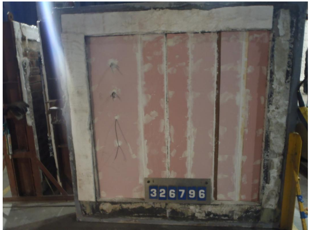
The exposed face of the wall construction prior to testing
