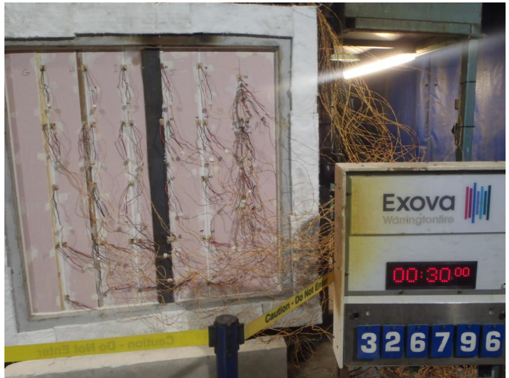
The unexposed face of the wall construction after 30 minutes of testing
