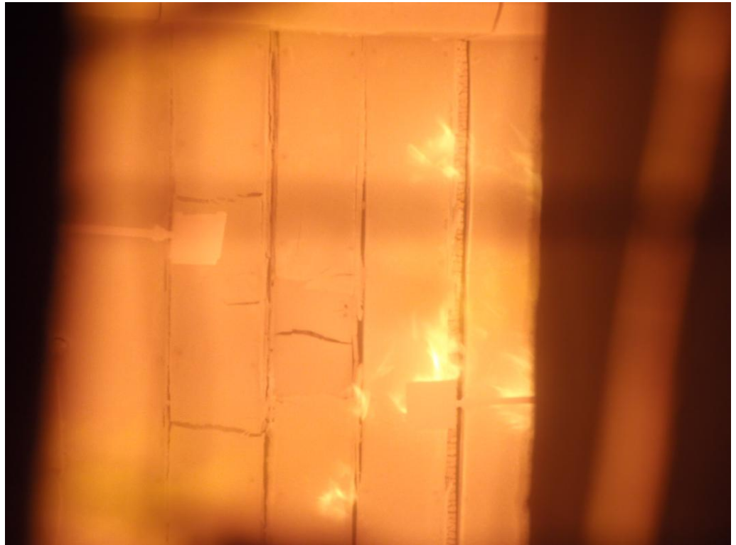
The exposed face of the wall construction after 90 minutes of testing
